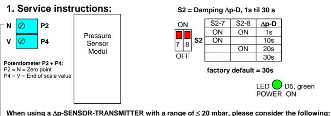
**Pot.** N = zero point. If the appliance has been transported and / or mounted not vertically (gravity influence on the sensor membrane), please adjust the zero point with P2 as soon as the operating temperature has been reached. Please make sure that the damping-switches S2-7 and S2-8 are in position ON = 1s, during the adjustment. With the **DIP-Switch S6**, on the right-hand side of terminal 13, the analogue output at terminal12 can be changed from 0-20 mA, S6 = ON to 4-20 mA, S6 = OFF.
