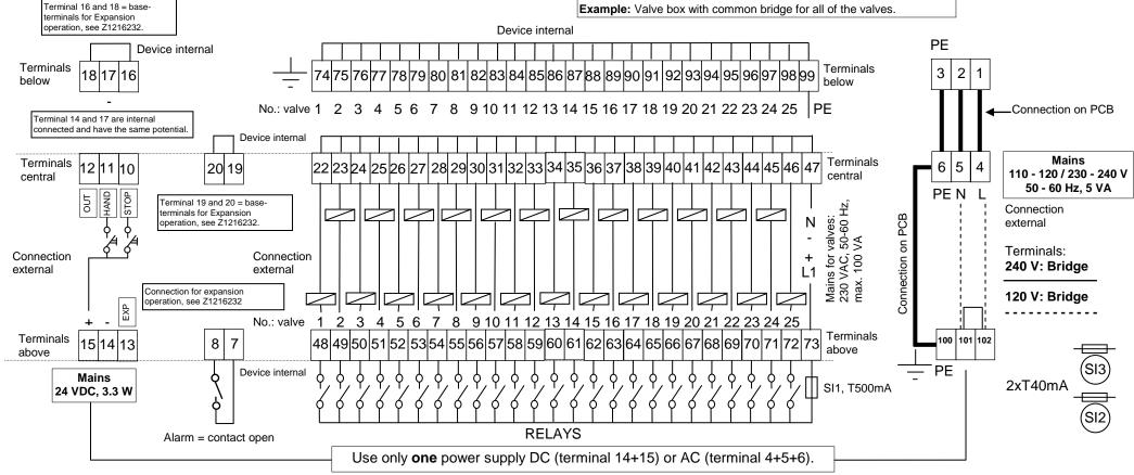
HAND - contact (external) closed: Cleaning with IMPULSE 1 and INTERVAL 1.
