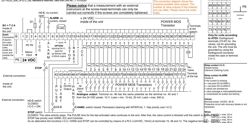
of the PLC must then be connected to terminal 45 (-24V).
