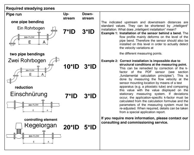
Take into account obstructions existing in front of and behind the selected mounting location. Passive elements (e.g. bends) cause less interference than active elements (e.g. fans). Harmonic changes in the pipe run (bends with large radii, reductions according to DIN) are more favourable than sudden or less harmonic changes (corners, stops). Contact the manufacturer or responsible sales engineer if necessary!
